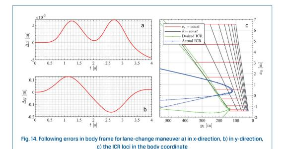
The ICR loci in the body coordinate is plotted and shown in Figure 14 (c). The transient nature of the manoeuvre is also observed in this figure. The ICR does not reach the desired (steady-state) location during the lane change, but the difference is small, proving the effectiveness of using a steady-state response as feed-forward and overall control performance, even for sudden manoeuvres.
