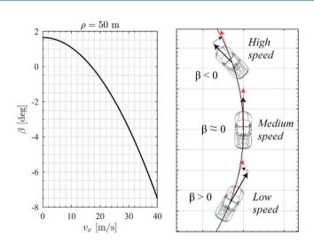
Fig. 3. Variation of side-slip angle versus velocity for a constant radius of curvature
